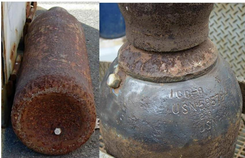
Small cylinders (MC and B) might only have the PRD drilled into the side of the valve.
