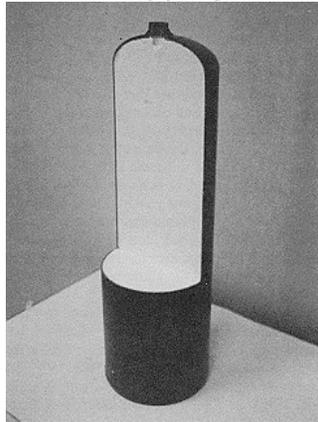
Most porous masses were previously made from asbestos since it is much more effective in controlling the decomposition due to superior physical characteristics. The porous mass is now made with a clay material with many microcavities. When a cylinder ruptures, all of the porous mass will be propelled out of the cylinder contaminating the area if it contained asbestos.
