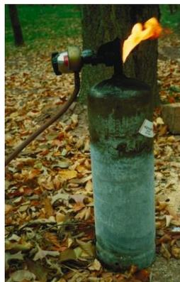
Cylinders in which the PRD has melted and the gas is on fire, should be allowed to burn in place. Never extinguish the fire. This will not be effective and could cause a safety problem due to an explosive environment being created. Even in open air, acetylene/air mixtures can detonate.
